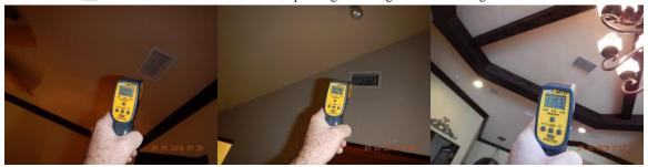
Infrared Thermometer was used to confirm the systems produced heat when operated during the Home Inspection
