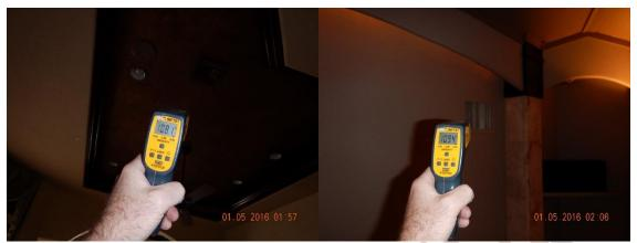
Infrared Thermometer was used to confirm the systems produced heat when operated during the Home Inspection
